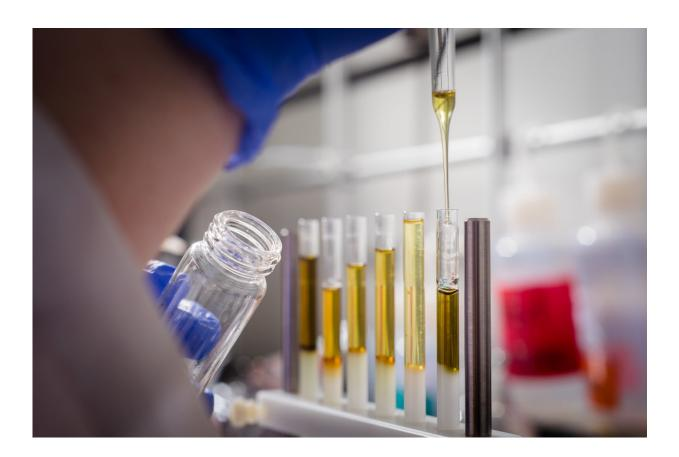
A researcher in the Organic and Stable Isotope Biogeochemistry Lab at UB, led by Assistant Professor of Geology Elizabeth Thomas, adds solvents to glass columns holding organic matter from lake sediment. This process enables scientists to separate out leaf waxes and bacterial lipids for further analysis. Though the samples shown here were not used in the new study, the methods depicted reflect the research team's procedures. Credit: Douglas Levere / University at Buffalo
