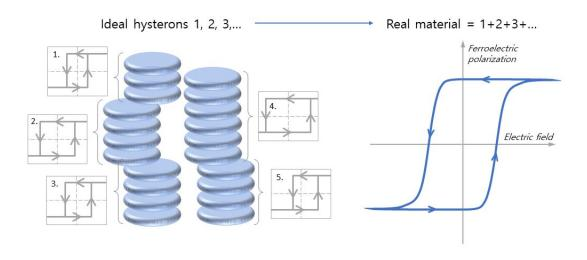
The organic ferroelectric material consists of nanometer-sized stacks of disk-like molecules that act as 'hysterons' with ideal ferroelectric behavior. Combined in a macroscopic memory device, the characteristic rounded-off hysteresis loop results. Credit: Indre Urbanaviciute och Tim Cornelissen
