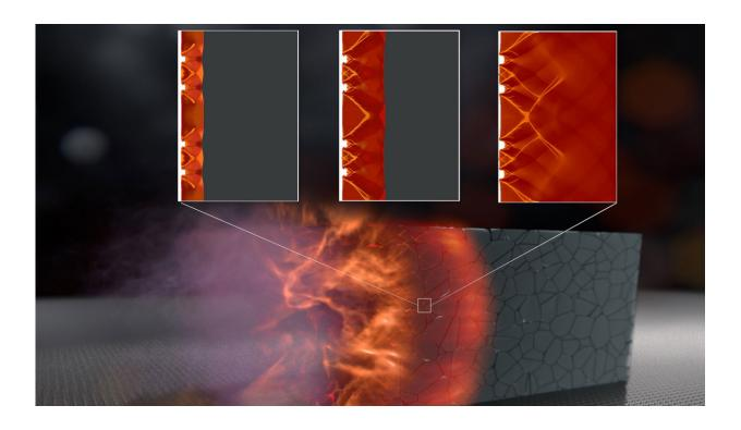
Supercomputer simulations of shock-induced explosive reactions suggest that the microstructure of heterogeneous solid explosive materials impact performance and safety. Credit: Lawrence Livermore National Laboratory
