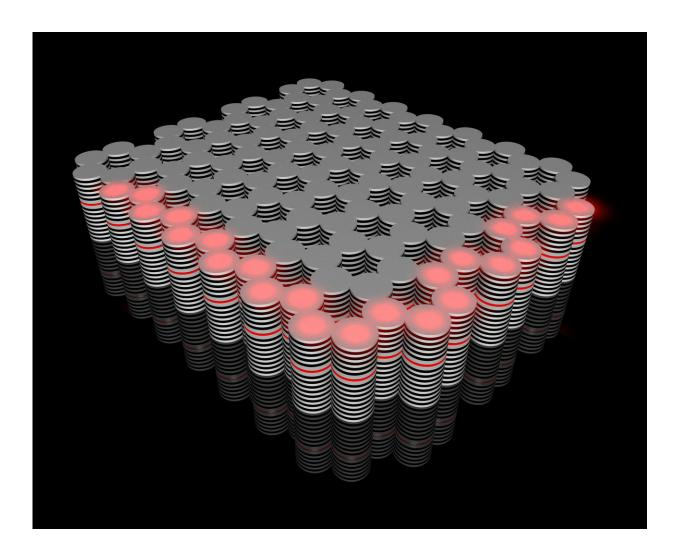
The novel topological insulator built in the Würzburg Institute of Physics: a controllable flow of hybrid optoelectronic particles (red) travels along its edges. Credit: Karol Winkler
