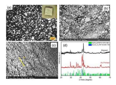
Images a) and b) show micrographs of additive manufacturing bonded magnet, after printing but before alignment. Figure c) shows a micrograph of the magnet after alignment, and Figure d) shows X-ray diffraction patterns comparing asprinted and post-aligned magnet samples. Credit: Ames Laboratory
