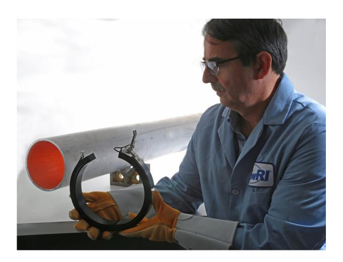
Dr. Sergey Vinogradov, an SwRI staff engineer and expert in sensor systems and nondestructive evaluation technology, holds the improved MsT device. The circular, hard-shell MsT sensor clamps around pipes and other metal and nonmetal structures and is available in a variety of circumferences. It detects material flaws, corrosion and areas at risk of developing breaks, cracks and leaks. Credit: Southwest Research Institute
