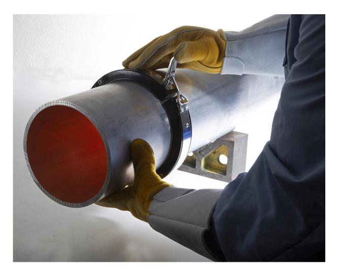
The user-friendly MsT sensor automatically adjusts frequencies to inspect structures, which reduces human error. At just 1.1 inches wide, MsT can squeeze into compact areas. The MsT can now scan a structure in segments, providing more precise and thorough inspections. Credit: Southwest Research Institute
