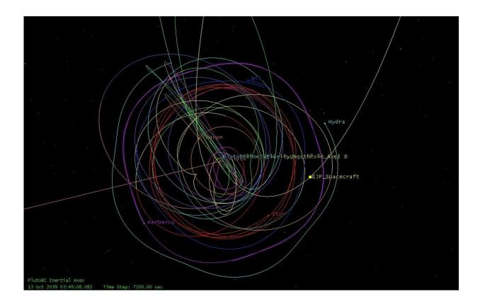
The SwRI-developed Pluto orbital tour design shows scientific objectives can be met with only tiny fuel resources and numerous gravity assists using Pluto's giant moon Charon. Credit: Southwest Research Institute
