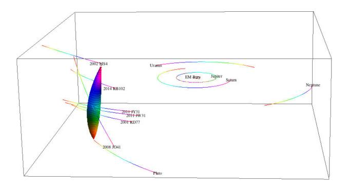
This figure depicts an electric propulsion spacecraft leaving Pluto orbit, flying by other small Kuiper Belt objects and then reaching the dwarf planet 2002 MS4 as just one example of the "gold standard" Pluto orbiter-Kuiper Belt explorer
