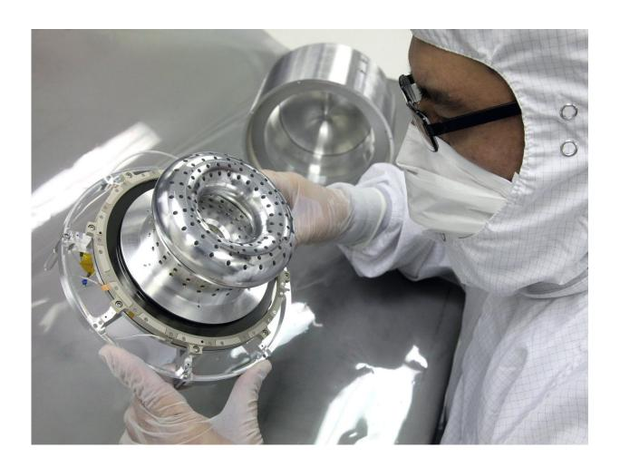
The ESA BepiColombo spacecraft bound for Mercury includes Strofio, an SwRI-developed novel spectrometer designed to measure the sparse particle population of the planet's tenuous exosphere. Development challenges included mass and configuration limits and operating in the harsh Mercury environment. Credit: Southwest Research Institute
