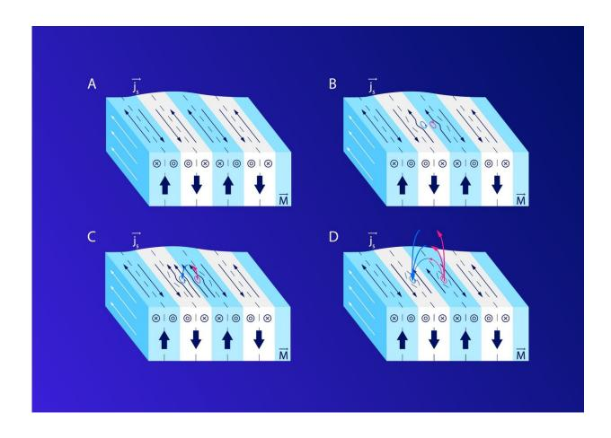
Below the ferromagnetic transition temperature, the material generates vortexantivortex pairs due to the effects of spontaneous screening Meissner currents. Thick arrows indicate the direction of the magnetization vectors, and thin arrows show the direction of the current. In the side view, a circle with a circle inside is a thin arrowhead, and a circle with a cross is a thin arrow end. Credit: Elena Khavina/MIPT
