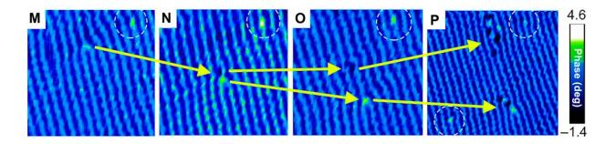
Cooling sample. The yellow arrows indicate the vortex-antivortex pair, as it is generated (N), separates (O), and further diverges (P). The authors note that the process is observed at domain junctions called Y dislocations (as in M) or on the site of a pre-existing vortex. Credit: Vasily Stolyarov et al./Science Advances
