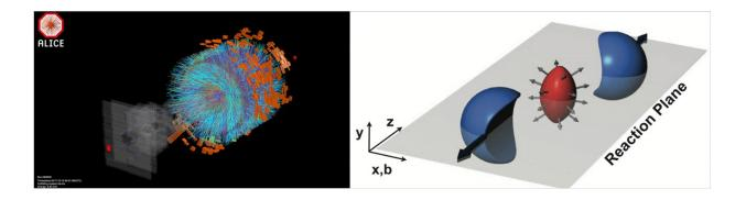
[Left] An event from the first Xenon-Xenon collision at the Large Hadron Collider at the top energy of the Large Hadron Collider (5.44 TeV) registered by ALICE [credit: ALICE]. Every colored track (The blue lines) corresponds to the trajectory of a charged particle produced in a single collision; [right] formation of anisotropic flow in relativistic heavy-ion collisions due to the geometry of the hot and dense overlap zone (shown in red color). Credit: University of Copenhagen
