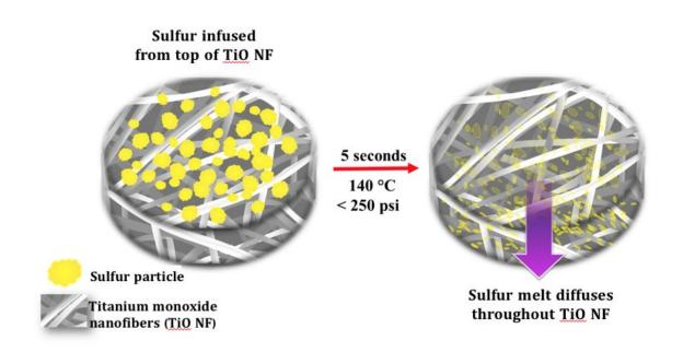
The hot-press procedure, developed at Drexel, melts sulfur into the nanofiber mats in a slightly pressurized, 140-degree Celsius environment -- eliminating the need for time-consuming processing that uses a mix of toxic chemicals, while improving the cathode's ability to hold a charge after long periods of use. Credit: Drexel University
