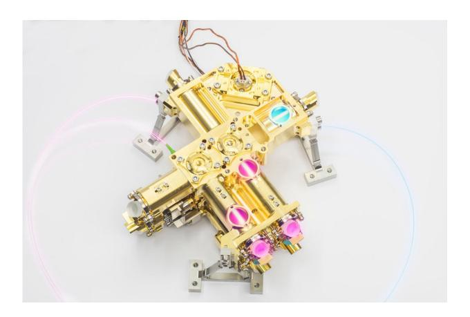
The quantum source generates entangled photons and transmits them to Earth from a satellite, where they serve to distribute secure keys for encrypting data. Credit: Fraunhofer IOF
