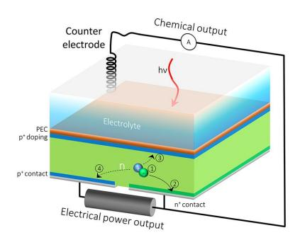
The HPEV cell's extra back outlet allows the current to be split into two, so that one part of the current contributes to solar fuels generation, and the rest can be extracted as electrical power. Credit: Berkeley Lab, JCAP
