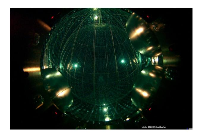
The Borexino instrument located deep beneath Italy's Appenine Mountains detects neutrinos as they interact with the electrons of an ultra-pure organic liquid scintillator at the center of a large sphere surrounded by 1,000 tons of water. Credit: Borexino
