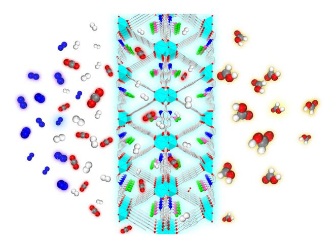
From the left, a mixture of gases, including CO2 (red and gray), N2 (blue), and H2 (white) are exposed to the nanoporous metal-organic framework designed by the Johnson group. Only the CO2 and H2 enter the MOF, which rejects the N2. The catalytic sites within the framework convert the CO2 to formic acid (red, gray and white), a chemical precursor to methanol Credit: Swanson School of
