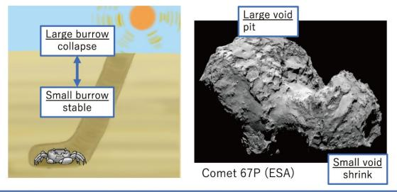
Size limits are determined by the stability of a void in cohesive granular matter
