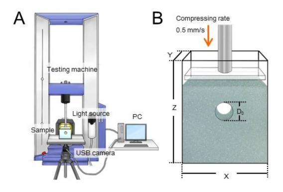
Tunnel compression experiment using a universal testing machine was performed in this study (A). A wet granular layer with horizontal tunnel structure was prepared in an acrylic vessel (B). The entire wet granular layer including the tunnel structure was uniformly compressed. Credit: Hiroaki Katsuragi
