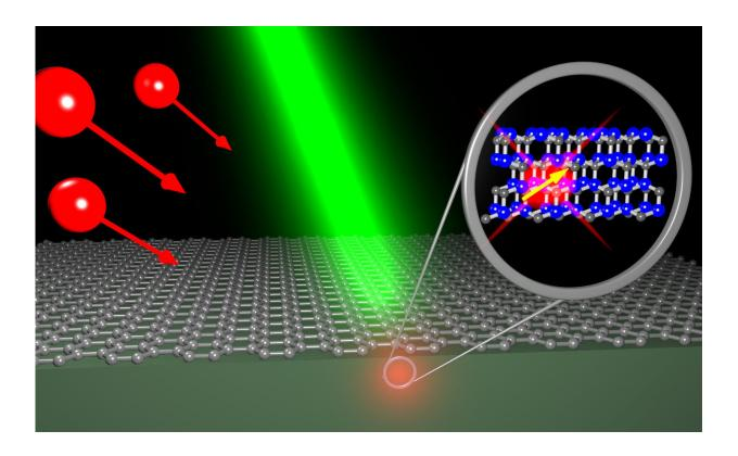
Green SiC substrate at the bottom with the graphene layer on top irradiated by protons, generating a luminescent defect in the SiC crystal. Credit: Maximilian Rühl
