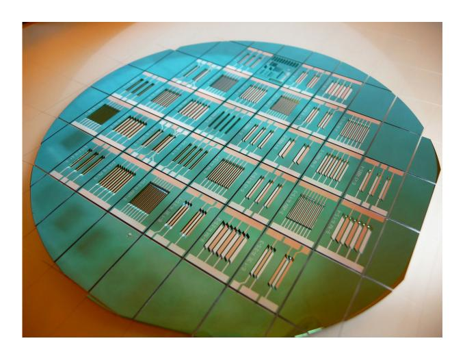
Fabrication of micro batteries with side-by side electrodes on silicon wafer. Credit: Fraunhofer IZM
