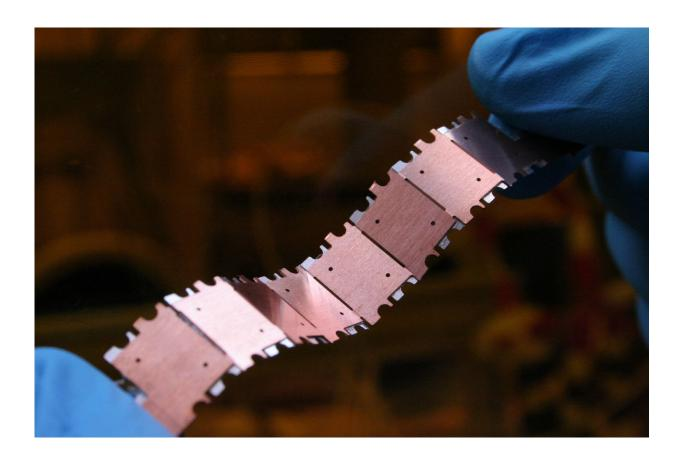
Mechanically flexible micro battery stripe made from segmented battery cells. Credit: Fraunhofer IZM
