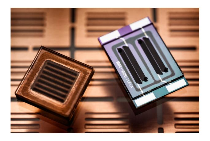
Millimeter-sized lithium-ion batteries with interdigital electrodes. Credit: Fraunhofer IZM, Volker Mai
