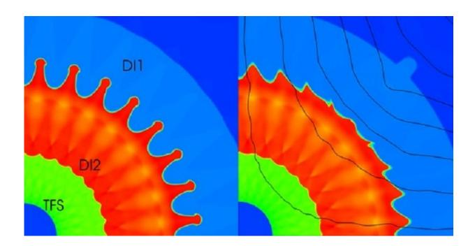
Computer simulations show that the Richtmyer–Meshkov instability (left) can be suppressed with a saddle-shaped magnetic field (right). Credit: *Matter and Radiation at Extremes*
