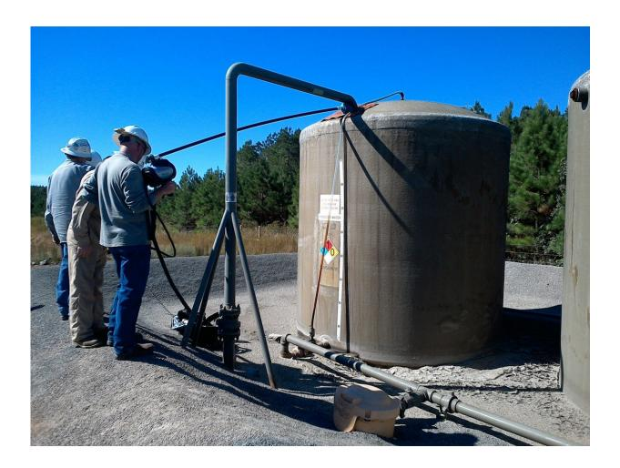
Operators measure methane emissions from a produced water tank at a gathering compressor station. Credit: Colorado State University
