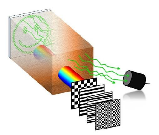
Laser light patterns are sequentially focused in time onto a region of interest inside biological tissue. Fluorescence emitted by the sample under each illumination pattern is collected with a single-pixel detector after passing back through the tissue. By adding up the projected patterns weighted by the intensities recorded, an image of the sample can be reconstructed. Credit: University of St Andrews
