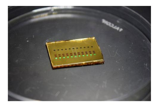
An array of 11 metasurface-based optical spectrometers, pictured here before the final fabrication step. Each spectrometer is composed of three metasurfaces that disperse and focus light with different wavelengths to different points. Credit: Faraon Lab/Caltech
