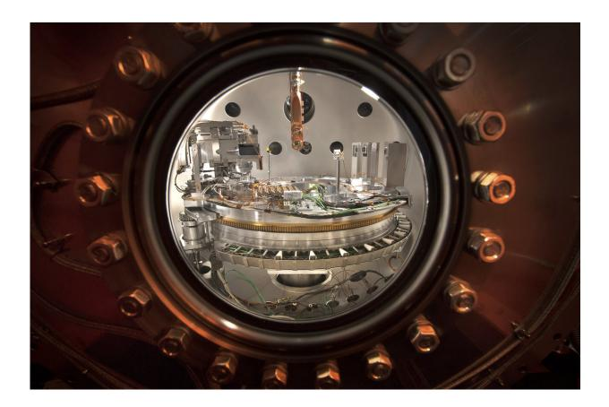
The sample chamber of the Soft Inelastic X-ray Scattering (SIX) beamline at NSLS-II allows scientists to mount their materials on a special holder that can be turned and moved into the beam of bright X-rays. Credit: US Department of Energy
