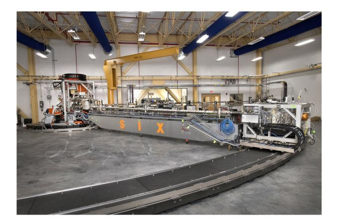
The Soft Inelastic X-ray Scattering (SIX) beamline at NSLS-II is notable for its 50-foot-long spectrometer arm that is housed in an adjacent building. The long, movable arm enables SIX to obtain an extremely high energy resolution and reveal the collective motion of electrons within a material. Credit: US Department of Energy
