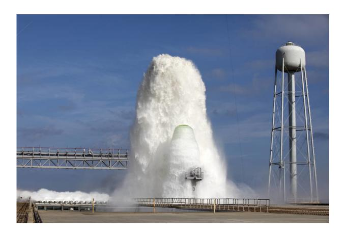
The IOP/SS system deploys almost a half-million gallons of water in one minute to protect the SLS during launch. Image Credit: NASA
