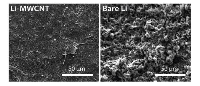
Microscope images of lithium metal anodes after 500 charge/discharge cycles in tests at Rice University show the growth of dendrites is quenched in the anode at left, protected by a film of carbon nanotubes. The unprotected lithium metal anode at right shows evidence of dendrite growth. Credit: Tour Group/Rice University
