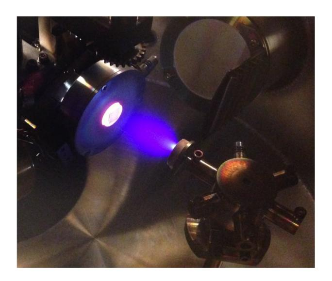
Inside view of the vacuum chamber in which the process of 'pulsed laser deposition' takes place, used to create the hafnium oxide crystals in this study. On the left the glowing substrate on which the film is growing with atomic control; in the center the blue plasma of ions that is created by shooting a laser on a target with the right chemical composition (target visible on the right side of
