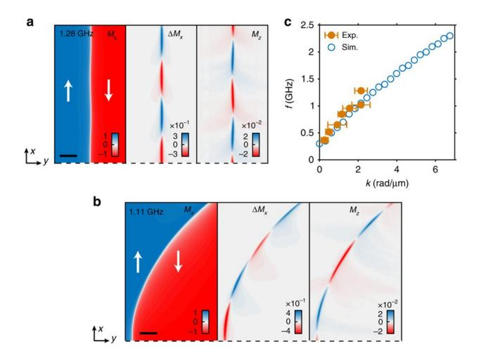
Spin-wave modes, simulated and experimental dispersion, a) micromagnetic simulations of the spin-waves mode in the presence of a straight Néel 1800 domain wall and in the presence of a curved Néel 1800 wall. The excitation was generated by a horizontal line antenna placed below the dashed line (the frequency is indicated in each panel). The arrows indicate the direction of magnetization within the domains, c) dispersion of the spin-waves confined at
