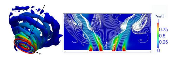
Left: Vortex structures of swirling flows. Right: Mixing pattern of two ammonia streams with the air stream near the swirlers, located at the bottom of the figure. Colours indicate ammonia mole fraction distribution, with higher amounts of ammonia molecules in red, and lower amounts in blue. Credit: Taylor & Francis
