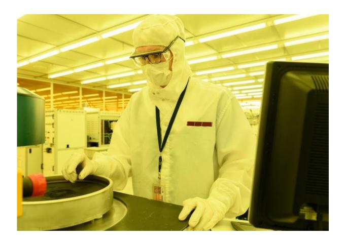
Georgia Tech graduate research assistant Mason Chilmonczyk examines a device after a plasma etch step in a reactive ion etching tool. The work was being done in the Institute of Electronics and Nanotechnology's Marcus Building clean room. Credit: Rob Felt, Georgia Tech
