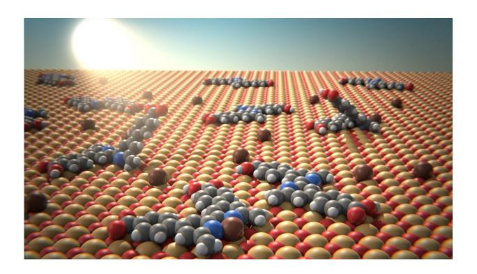
Scientists were able to determine the spatial arrangement of bipyridine molecules (gray) on a surface of nickel and oxygen atoms (yellow/red). Rotation changes the transconfiguration (front right) to a cis configuration (front left). Credit: University of Basel, Department of Physics
