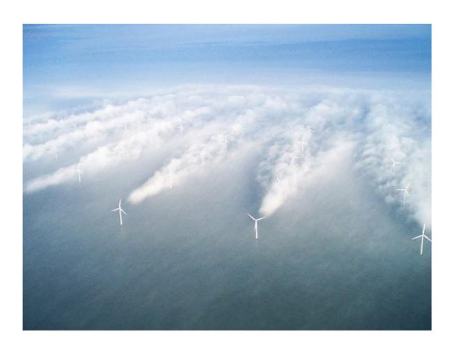
Fog at an offshore windfarm shows the formation of wind shadows between wind turbines. Credit: VATTENFALL
