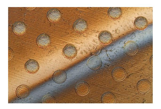
This photo shows circles on a graphene sheet where the sheet is draped over an array of round posts, creating stresses that will cause these discs to separate from the sheet. The gray bar across the sheet is liquid being used to lift the discs from the surface. Credit: Felice Frankel
