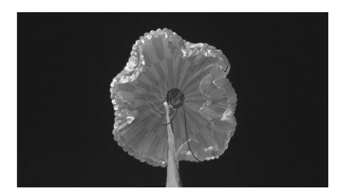
This high-definition image was taken on Sept. 7, 2018, during the third and final test flight of the ASPIRE payload. It was the fastest inflation of this size parachute in history and created a peak load of almost 70,000 pounds of force. Credit: NASA/JPL-Caltech
