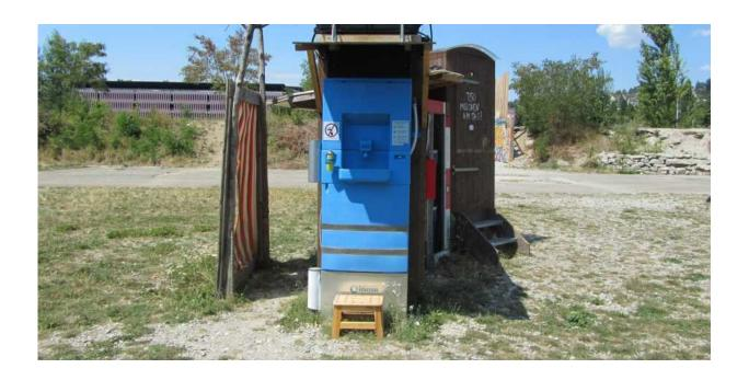
Local water treatment: The recycling plant for slightly contaminated wastewater in the field test in summer 2018 in the Hardturm Stadionbrache in Zurich. Credit: Eva Reynaert/Eawag
