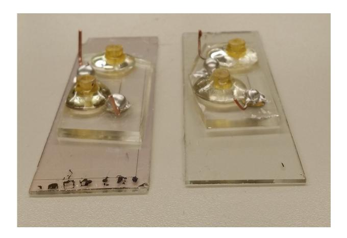
Lab-on-a-chip devices harness electrical signals to measure glucose, tell apart blood type and detect viruses or cancer. But biological samples need protection from the electric fields. A thin layer of hafnium oxide does the trick. Credit: Sanaz Habibi
