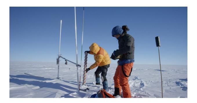
Coring next to a stake assembly of the Q-transect station network. The station records snow height, but we need to measure the weight of the snow to use these
