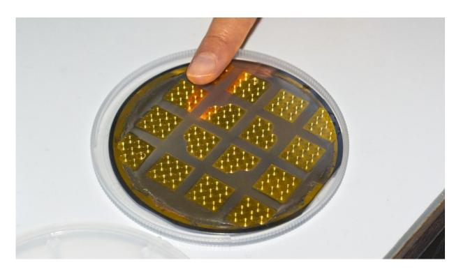
The watch springs are electroplated on a gold plated silicon wafer, coated with a light-sensitive paint. Credit: Empa
