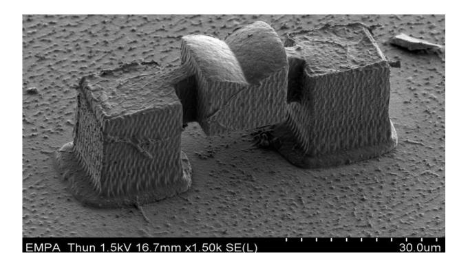
The team succeeded in producing bridges and columns made of solid nickel that are only a few micrometers in size. Credit: Empa
