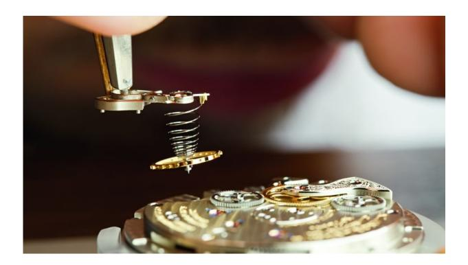
The balance wheel is the beating heart of every mechanical watch mechanism. The delicate springs are usually made of cast, forged Nivarox alloy. At Empa a new generation of balance springs is produced with means of electroplating. Credit: A. Lange & Söhne
