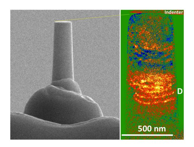
Dislocation avalanche in a high entropy nanopillar. Focused ion beam is used to fabricated the nanopillar (left) for compression test. Transmission electron microscope is used to image dislocation pile up during a dislocation avalanche (see D on the right). Credit: Frederick Seitz Materials Research Lab
