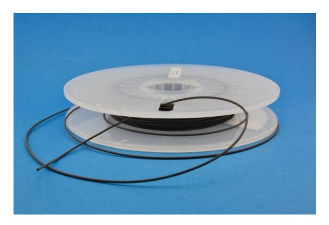
Flexible filament consisting of a polymer-magnetic powder mixture. Credit: Kai von Petersdorff-Campen / ETH Zurich
