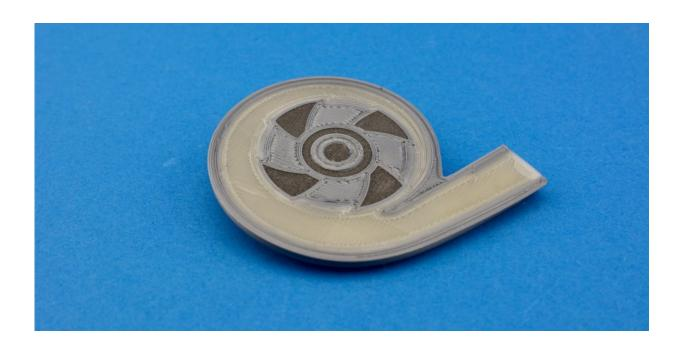
Cross section of the prototype. The dark grey magnetic components are clearly visible. Credit: Kai von Petersdorff-Campen / ETH Zurich
