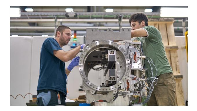
A new beam absorber for the zones where the beams are injected from the SPS was assembled and tested last summer. This is one of the developments presented at the High-Luminosity LHC annual meeting. Credit: Julien Ordan
