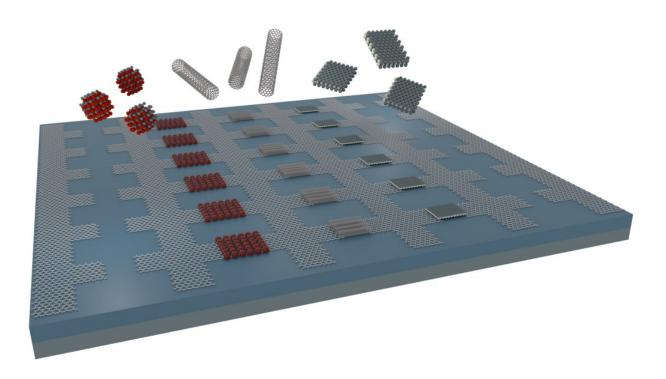
Artistic rendering of electric field-assisted placement of nanoscale materials between pairs of opposing graphene electrodes structured into a large graphene layer located on top of a solid substrate. Quantum dots (red), carbon nanotubes (grey), and molybdenum disulfide nanosheets (white/grey) are shown as representative 0D, 1D, and 2D nanomaterials that can be assembled at large scale based on the graphene-based, electric field-assisted placement method. Credit: IBM
