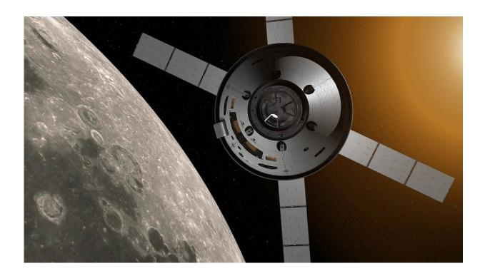
The ATV-derived service module, sitting directly below Orion's crew capsule, will provide propulsion, power, thermal control, as well as supplying water and gas to the astronauts in the habitable module. The first Orion mission will be an uncrewed lunar flyby in 2017, returning to Earth's atmosphere at 11 km/s – the fastest reentry ever. Credit: NASA
