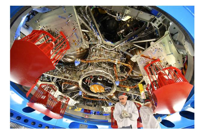
Technicians work underneath the European Service Module for NASA's Orion spacecraft, September 2018. Credit: ESA–A. Conigli
