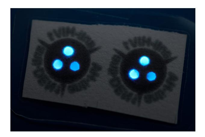
This paper strip (extremely zoomed in) contains two copies of the test. The three glowing dots per test indicate that you can check on three different antibodies within one test. Credit: Bart van Overbeeke
