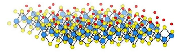
Fluoridating two-dimensional tungsten disulfide adds metallic islands to the synthetic semiconductor, along with unique optical and magnetic properties, according to researchers at Rice University. Credit: Ajayan Research Group/Rice University
