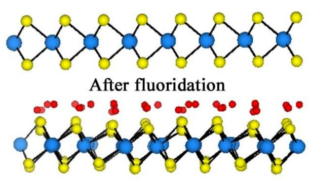
Fluoridating two-dimensional tungsten disulfide adds metallic islands to the synthetic semiconductor, along with unique optical and magnetic properties, according to researchers at Rice University. Credit: Ajayan Research Group/Rice University
