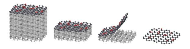
They are formed by ultrathin layers, held together by weak bonds, thus it is possible to control their thickness by simple peeling. The magnetic properties are given by the spin, represented with red arrows. Credit: IBS
