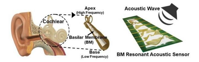
A flexible piezoelectric acoustic sensor mimicking the human cochlear. Credit: KAIST
