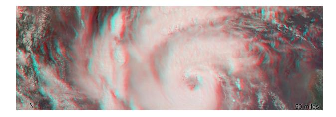
MISR's stereo analyph shows a three-dimensional view of Michael and combines two of MISR's nine camera angles. Using 3D red-blue glasses, you can see the 3D effect. Apparent in the 3D stereo analyph as well as the height field are a number of bright "clumps." These are groups of strong thunderstorms embedded within the larger circulation of the hurricane. Credit: NASA/GSFC/LaRC/JPL-Caltech, MISR Team
