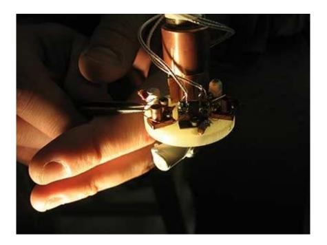
Ames Laboratory has developed a method to measure magnetic properties of superconducting and magnetic materials that exhibit unusual quantum behaviorat very low temperatures in high magnetic fields, by placing a tunnel diode resonator, an instrument that makes precise radio-frequency measurements of magnetic properties, in a dilution refrigerator, a cryogenic device that is able to cool samples down to milli-Kelvin temperature range. Credit: Ames Laboratory, US Department of Energy
