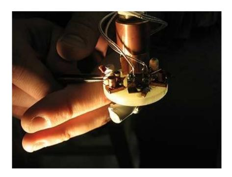
Ames Laboratory has developed a method to measure magnetic properties of superconducting and magnetic materials that exhibit unusual quantum behaviorat very low temperatures in high magnetic fields, by placing a tunnel diode resonator, an instrument that makes precise radio-frequency measurements of magnetic properties, in a dilution refrigerator, a cryogenic device that is able to cool samples down to milli-Kelvin temperature range. Credit: Ames Laboratory, US Department of Energy
