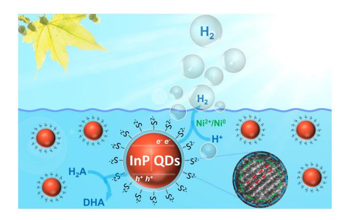
Schematic representation of photocatalytic hydrogen production with InP/ZnS quantum dots in a typical assay. Credit: Shan Yu
