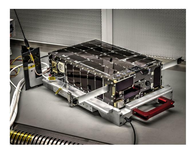
The tiny 6U (or six cubic units) Dellingr CubeSat, seen here in the lab before launch, carries two magnetometers designed to measure Earth's magnetic fields and an instrument called the Ion Neutral Mass Spectrometer, or INMS. INMS was designed to measure both the ions and neutral particles in Earth's ionosphere, a volatile region of the atmosphere that expands and contracts in response to the electrifying influence of the sun. Credit: NASA
